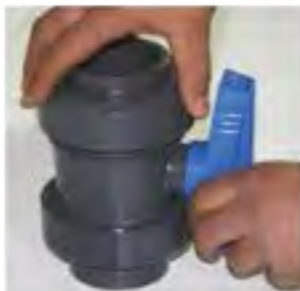
The union nut on the bush side is turned clockwise and removed. Union nut and pipe connection is removed.
