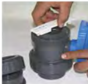
Ring is opened by turning counter clockwise.
