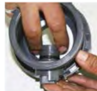
Pin is pulled from outside to inside and removed. It is held by the other hand at inside. Pin is taken out after removed.
