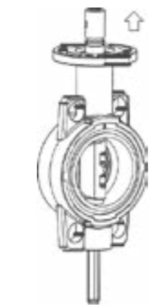
8. Turning square mil 15°, insert it inside through the bottom part of the valve and remove the sealed step above by pushing.
