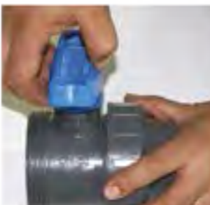
Handle is pulled and removed from the valve.
