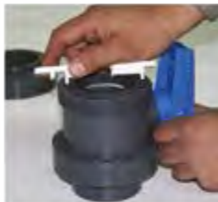
Teeth beneath the handle cover are placed their slots on the tightening component bearing (ring).
