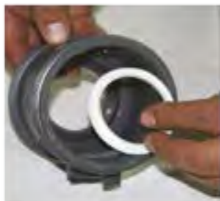
Ball inside casing is taken out together with its seal ring.
