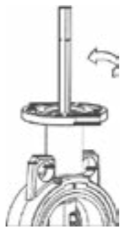
6. Pull back the square mil up to the level of the sealed step above. In order to remove the sealed step above before taking out the square mil, Turn the top step up to 30° degrees.
