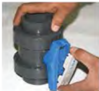
Handle cover of ball valve is pulled and removed by holding it on the groove.
