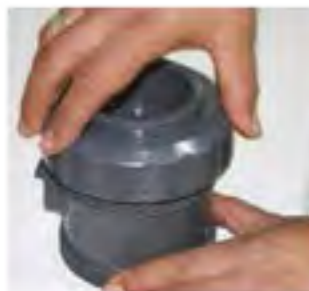
The union nut on the casing side is turned clockwise and removed.
