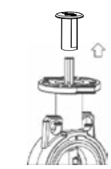
5. End stop is on the square mil, remove end stop.
