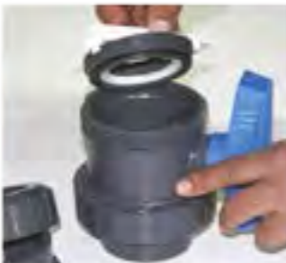
When ring threads are detached from the body, it can be removed with the lever lid.
