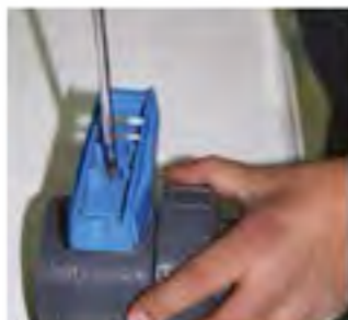
The screw on the handle is removed with a screwdriver.
