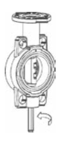
10. Turn the square mil up to 30° degrees to remove the square mil. Turn the square mil and disc 30°, remove the square mil from the valve completely.
