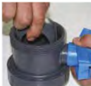
Ball is held with fingers on both edges and removed. Here, ball can be pushed on the bottom to support the removing force.
