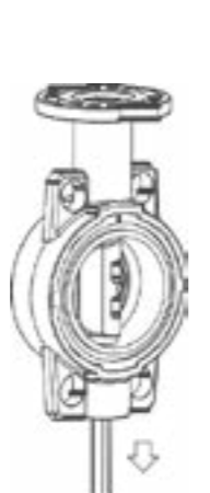
9. After removing the sealed step, take out the square mil from the bottom. Pull back the square mil to the level of sealed step.
